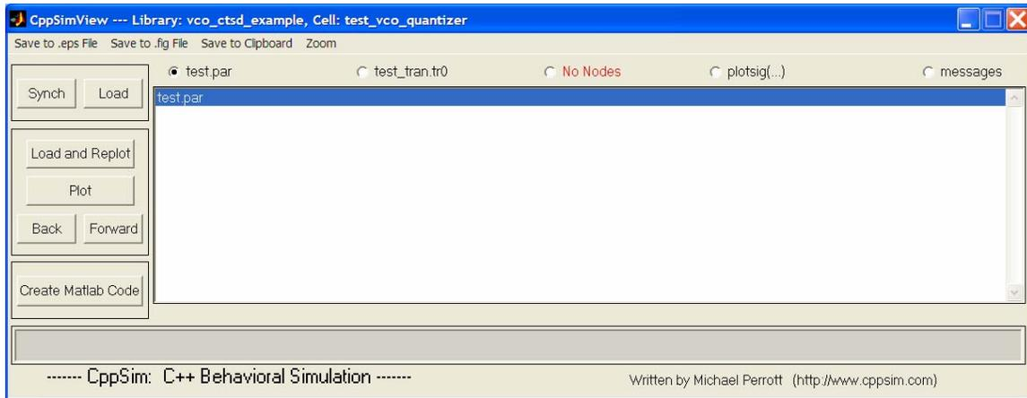
To view the simulation results, first click on the radio button titled **No Output File**. Immediately after this button is clicked, the radio button will instead display the output file's name, **test\_tran.tr0**. Next, click on the Load button on the left-hand side of the CppSimView window. Once this button is pressed, the **Nodes** radio button will be filled in, and the probed nodes will be listed, as shown below.
